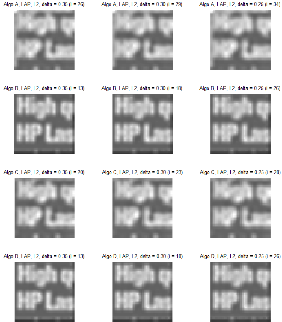
Figure 4.33: Reconstructed images of the real frames set 1 ( \delta = \text{RMSE} between the reconstructed images, i = \text{iteration} , A is for the "Classical SRR algorithm", B the "Fast SRR algorithm based on Recursive Least Square", C the "SRR algorithm based on Simultaneous Image Registration" and D the "Proposed SRR algorithm")
